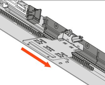
Fitting the driver pins to the runners
