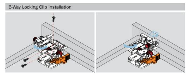
Remove screw on top adjustment arm and pivot out of the way. Fix the locking device onto the drawer bottom using two screws. Swing the adjusting part back into place and retighten holding screw.
