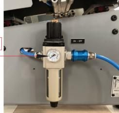
If the machine does not seem to be working properly, make sure the valve is located on the ON position.
