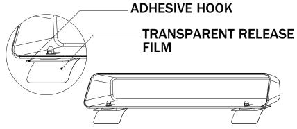
Tear the transparent release film off the adhesive hook.
