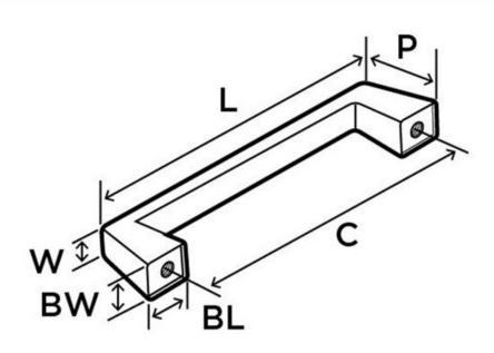
L (Length) = 5-15/16in(151mm) W (Width) = 1/2in(13mm)
