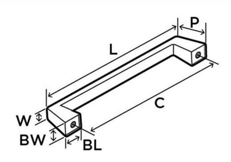
L (Length) = 7-1/4in(184mm)W (Width) = 1/2in(13mm)
