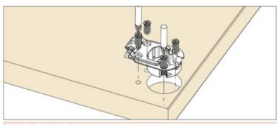
Deploying the system to the cups Connecting the system to the cups. This operation is tool free.
