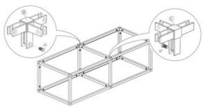
Advanced Assembly with 5-Way Corner Connectors
