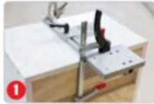
1 Clamp jig in desired location.
