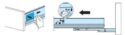
To re-install, place drawer on extended slides and push the drawer in fully. When it clicks, the lock will be engaged. Replace cover caps on both sides.
