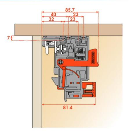
6-Way Adjustable Clip shown in diagram. Position the left and the right clip at the front of the drawer. Fix with the screws on the bottom or on the front of the drawer.
