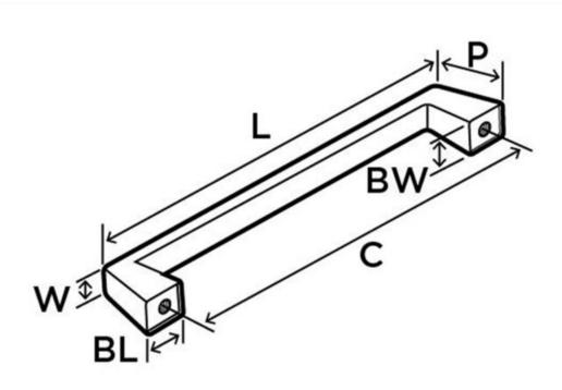
L (Length) = 9-3/8in(238mm) W (Width) = 3/4in(19mm) P (Projection) = 1-11/16in(43mm)
