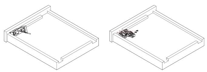
Mark the position of the locking device and fix the locking device onto the drawer. Drill holes on the back panel.
