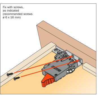
Use drilling template ASGD704U3XA for accurate installation of the clips, see page 51.
