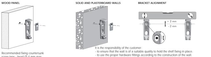
Recommended fixing countersunk screw type - head  $\breve{O}$  4 mm max.
