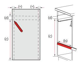
Measure the cabinet width (b), and the runner hole height (c), and spacing (d), mark on the door.
