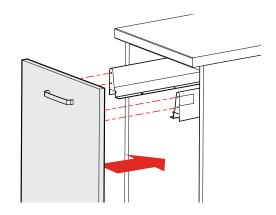
Mount door runner brackets to door and clip into the runners.
