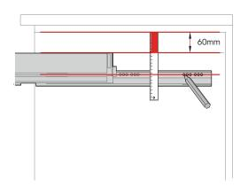
Measure 60mm (minimum) to top of runner and mark location of mounting holes.
