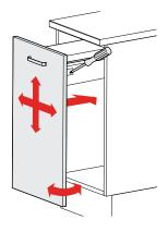
Re-install drawer assembly and adjust door.
