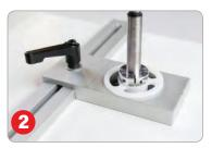
Drill light hole to desired depth using adjustable stop.
