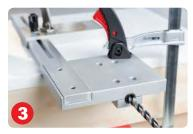
Leave clamps in place drill wire hole until bit reaches light hole.
